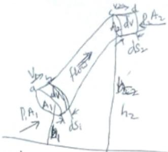
Caution: Bernoulli's eqn is valid for only incompressible steady flow of a fluid with no internal friction.
